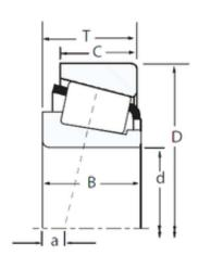
32215 Bearing 2D drawings and 3D CAD models
